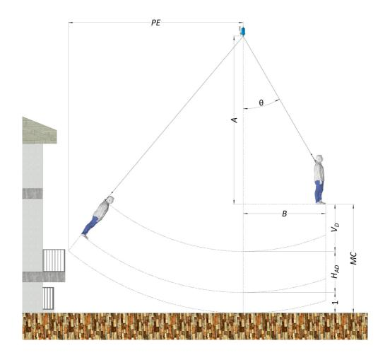
30 29 27 28 10 11 12 13 14 15 16 17 18 19 20 21 22 23 24 25 26 MINIMUM Fall and Pendulum Swing Clearance at MAXIMUM Lateral Offset LINE EXTRACTION/WORK POSITION A (METRE) Minimum Clearance (MC) & Pendulum Effect (PE) at Maximum Lateral Offset (B) Graph 16 DISTANCE (METRE)
