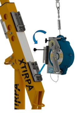
Remove the locking pin from the arrester bracket. Hook the arrester bracket onto the interface plate of the davit, rotate into place and replace the pin.
